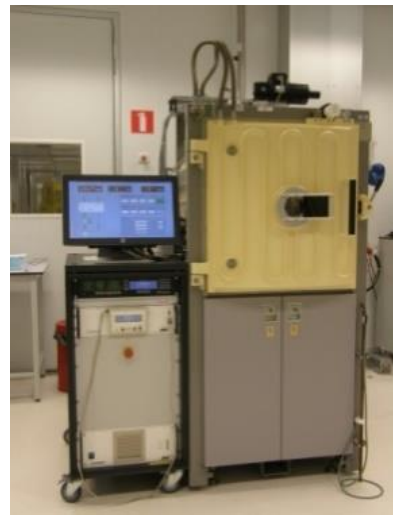
Figure 3.3. Focused electron beam (e-beam) vaporization source [4] and photograph of the BAK 600 e-beam evaporation system in the MESA+ cleanroom.
