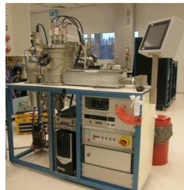
Figure 3.2 Illustration of the magnetron sputtering process [2] and photograph of the magnetron sputtering system 'Sputterke' in the MESA+ cleanroom.
